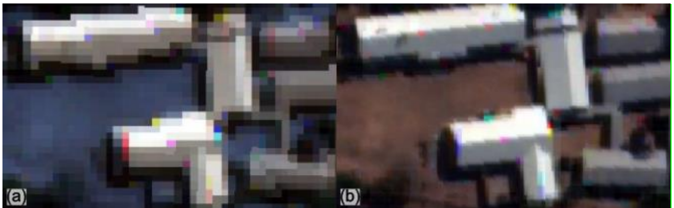
Figure 3. WorldView-2 satellite images (a) RGBNIR image and (b) pan-sharpened image
