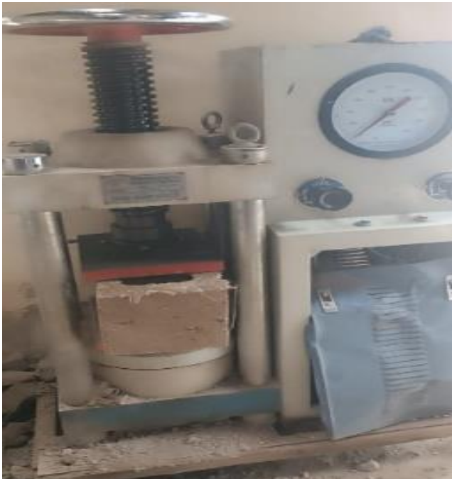
Figure 2. Compressive strength test
