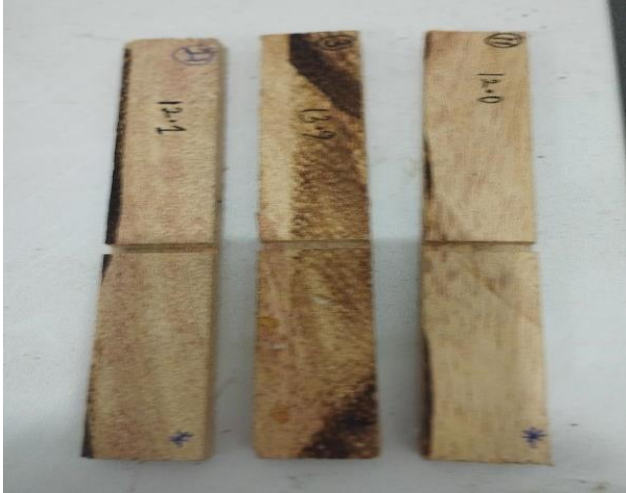
Figure 3. Resized, glued joints specimen.
