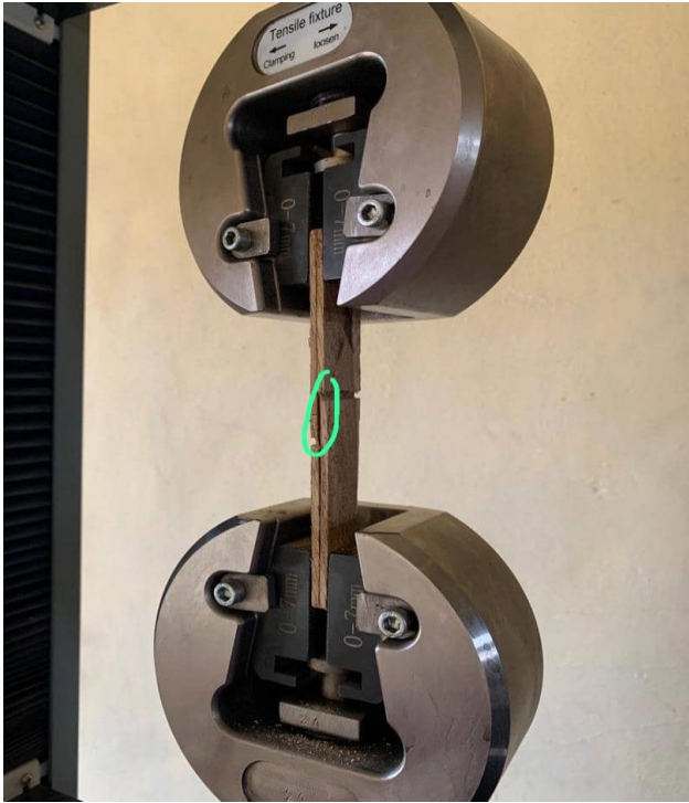
Figure 10a. glued joint between tensile loading jaw
