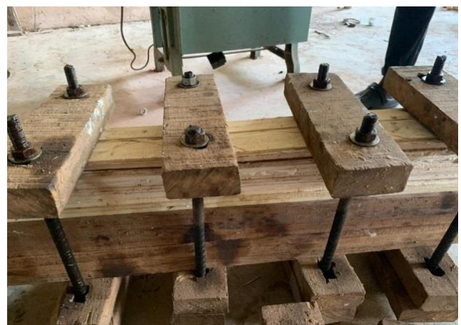
Figure 2. Clamping of laminates
