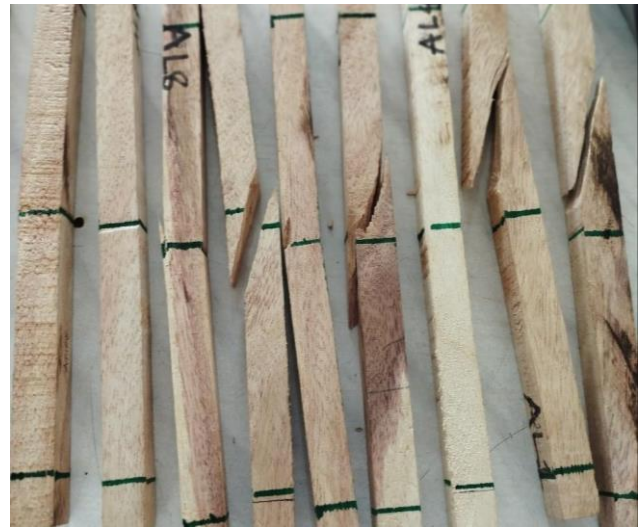
Figure 4: Samples after bending strength test
